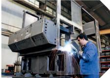
Final assembly in the new assembly plant tailored to special-purpose machinery construction
