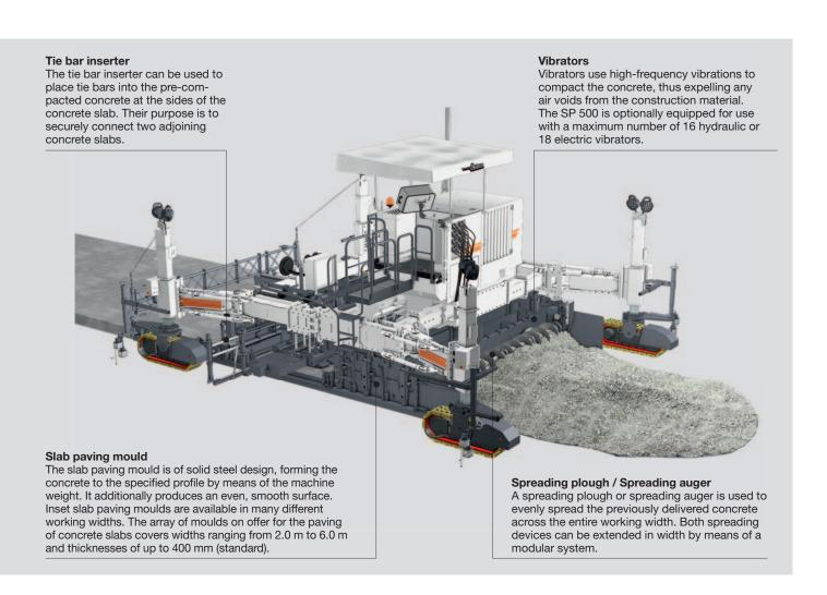
concrete paving of country roads, motorways, airports, railway tracks and all kinds of concrete profiles.
